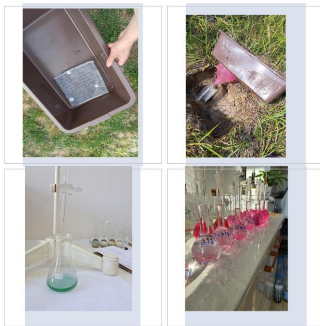
Figure 1. Lysimeter installation and laboratory procedures used for soil-water collection and chemical analysis.
