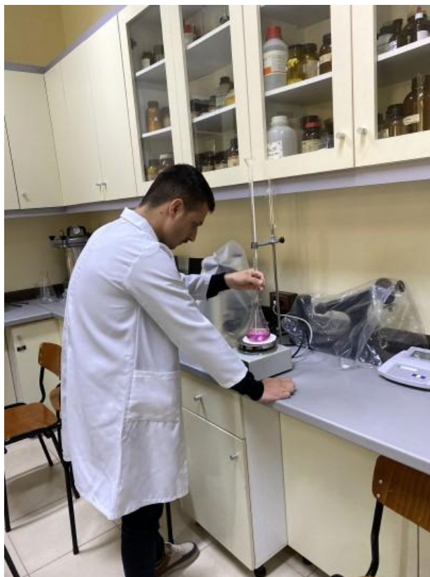
Photo 1. Titration process, recording the general hardness results converted to German degrees
