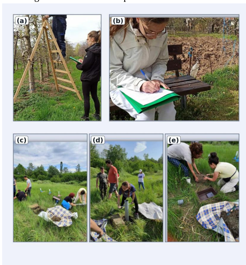
Figure 1. Fieldwork and experimental setup in the Ezerani wet meadow: (a-b) farmer interviews and questionnaire administration; (c-e) excavation and installation of plastic lysimeters.
