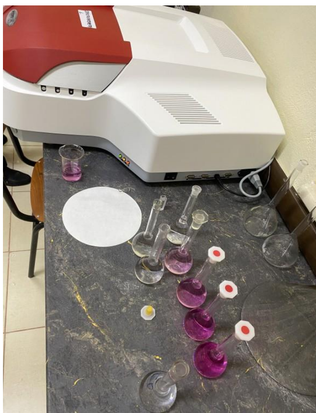
Photo 2. Measuring nitrite content in water with the spectrophotometer
